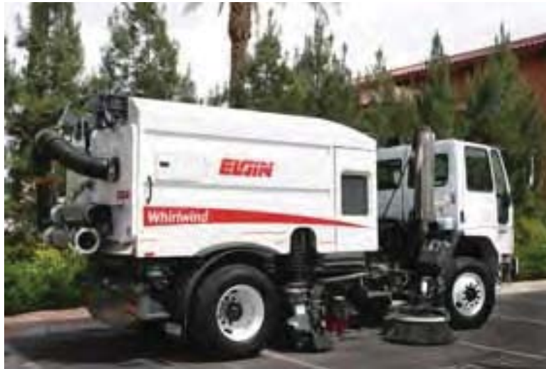
Figure 3: Photo of Elgin Whirlwind Vacuum Air Sweeper, example of effective vacuuming device
