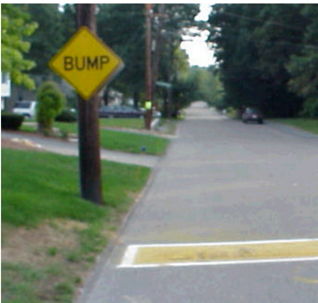
EXHIBIT 15 Speed bumps on Fox Hill Road in Burlington, a residential street leading to a school. There are 7 bumps within a 1.25 miles. These bumps are not as effective as Weston's because they do not extend to the edge of road. Drivers can swerve so that only their left tires hit the bump.
